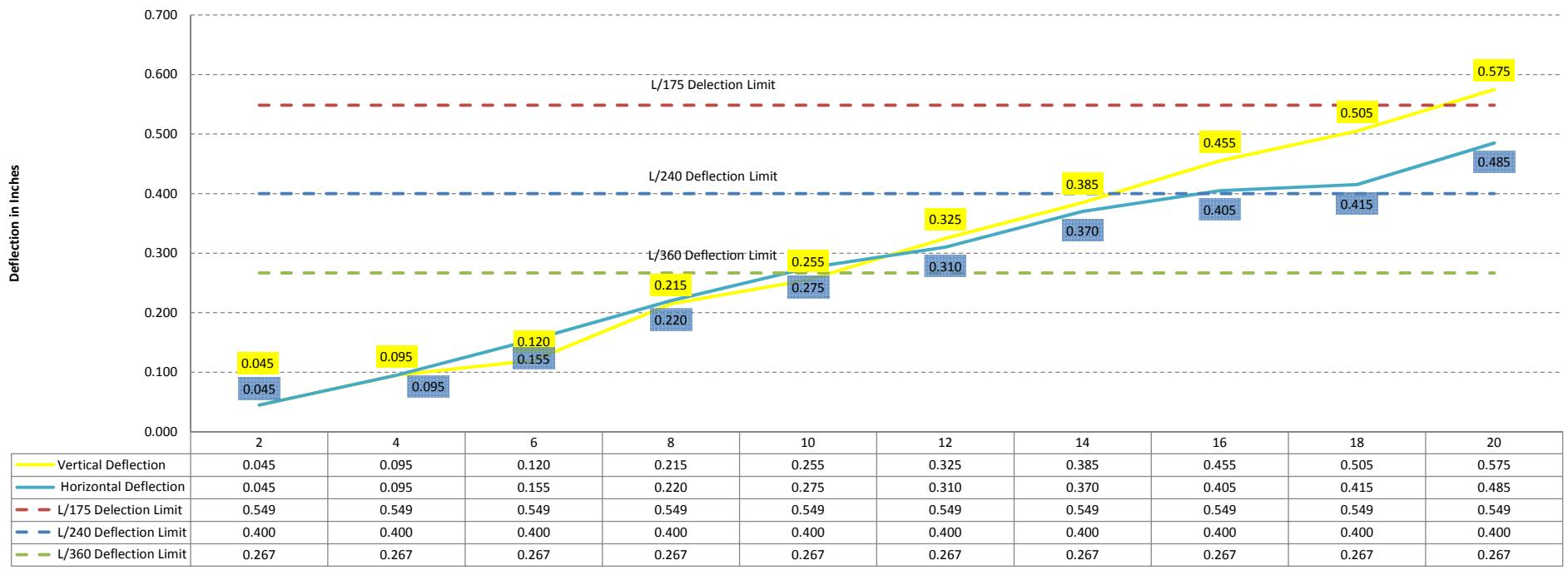
Units were tested 20 gauge galvanized skins on both sides
