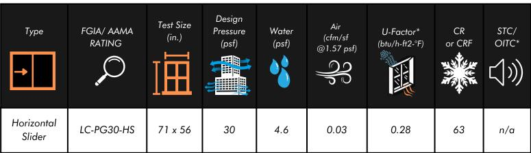
\*Performance varies based on glass selection, contact WinTech for project specific performance. U-Factor based on 3/4" IGU with soft-coat low-e and argon.
